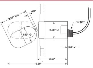
TK1 with flanged connection and SPST or SPDT switch with flying leads
